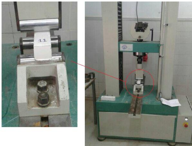
Fig. 8. Sketch of Device for the three-point bending strength test
