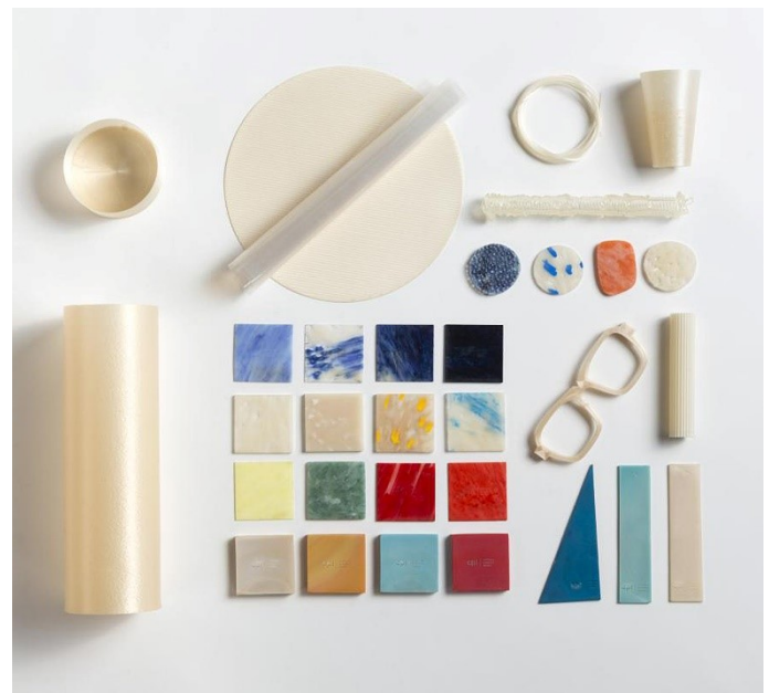
Figure 11: Samples of bioplastic Nuatan processed by various technologies. © Crafting Plastics studio Source: https://www.craftingplastics.com
