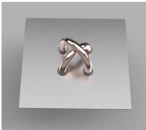
Fig. 4 3D model of the pressductor with the magnetizing and sensing coils. The coils are modeled as one single, homogenous turn of wire
