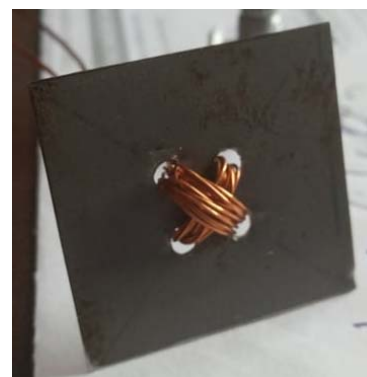
Fig. 9 Pressductor sensor sheet with the magnetizing and sensing winding
