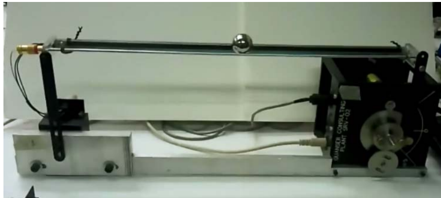
Figure 1 Ball and beam system
