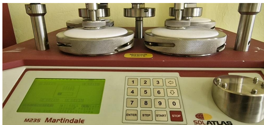
Figure 2. The Martindale pilling test made for the two products analyzed
