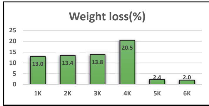
Figure 1. Weight loss (%) of dry nonwoven samples under UV light
