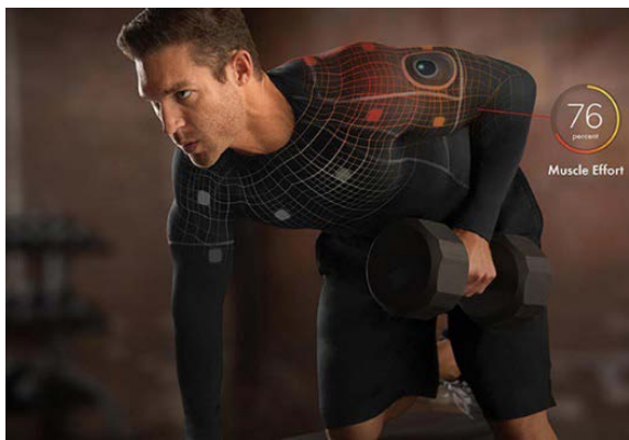
Figure 5 – Athos, smart clothing system using electromyography [42].
