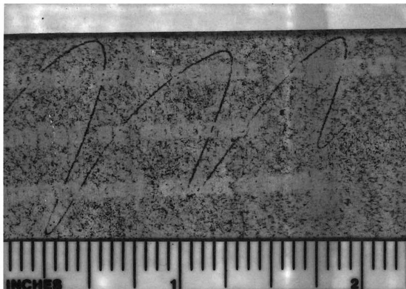
Figure 4. ESDA lift of laser printing over impressions.
