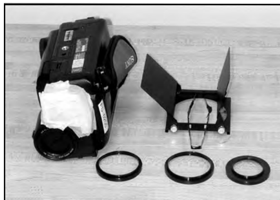
Figure 6. Modified Sony camcorder with step-up rings and filter holder
