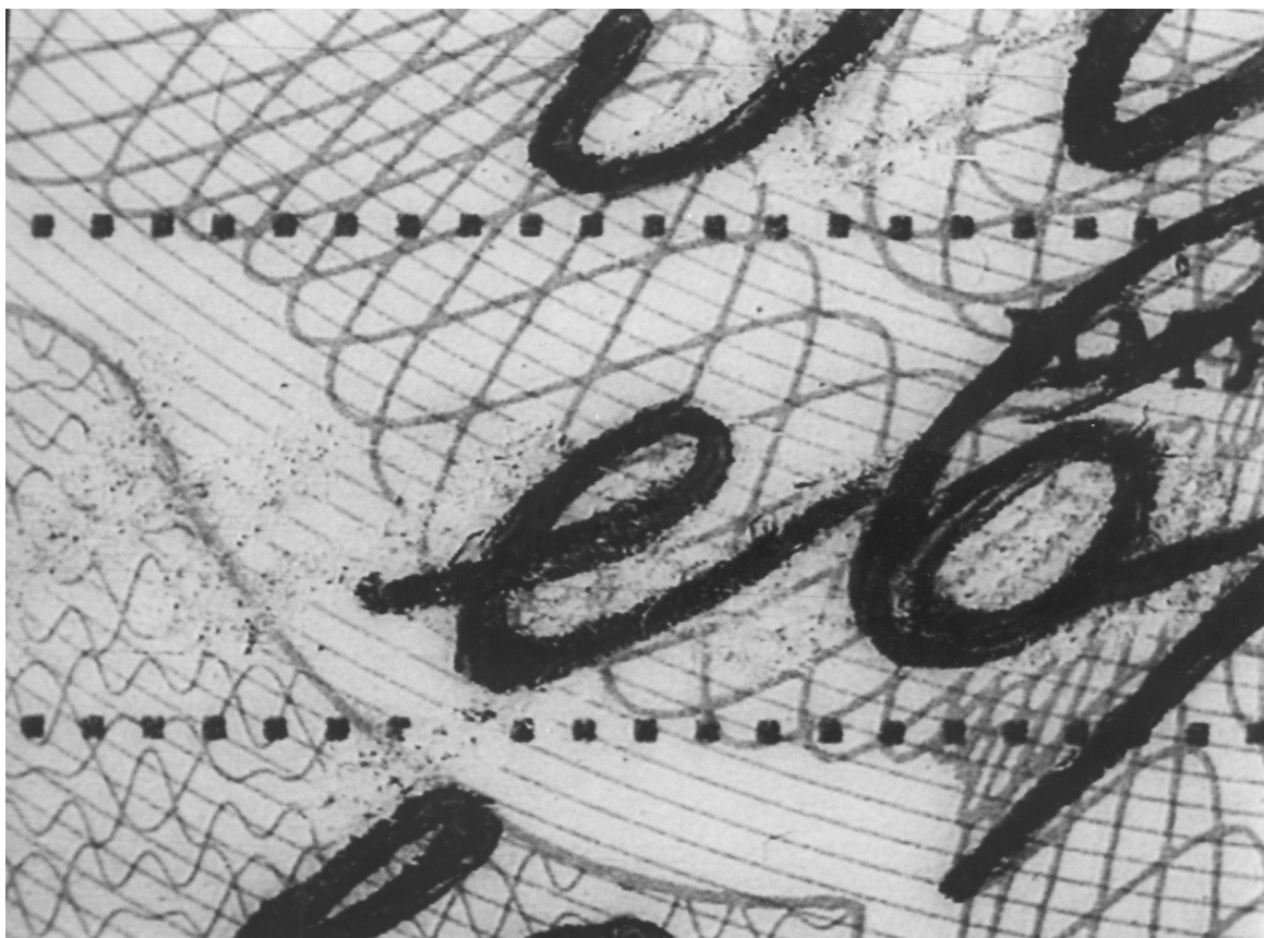
Figure 10. Fine mechanical erasure of handwritten entries on a USSR document.
