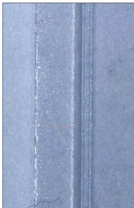
Figure 3 Ultrasonic welding used for sealing long edge of sleeve.
