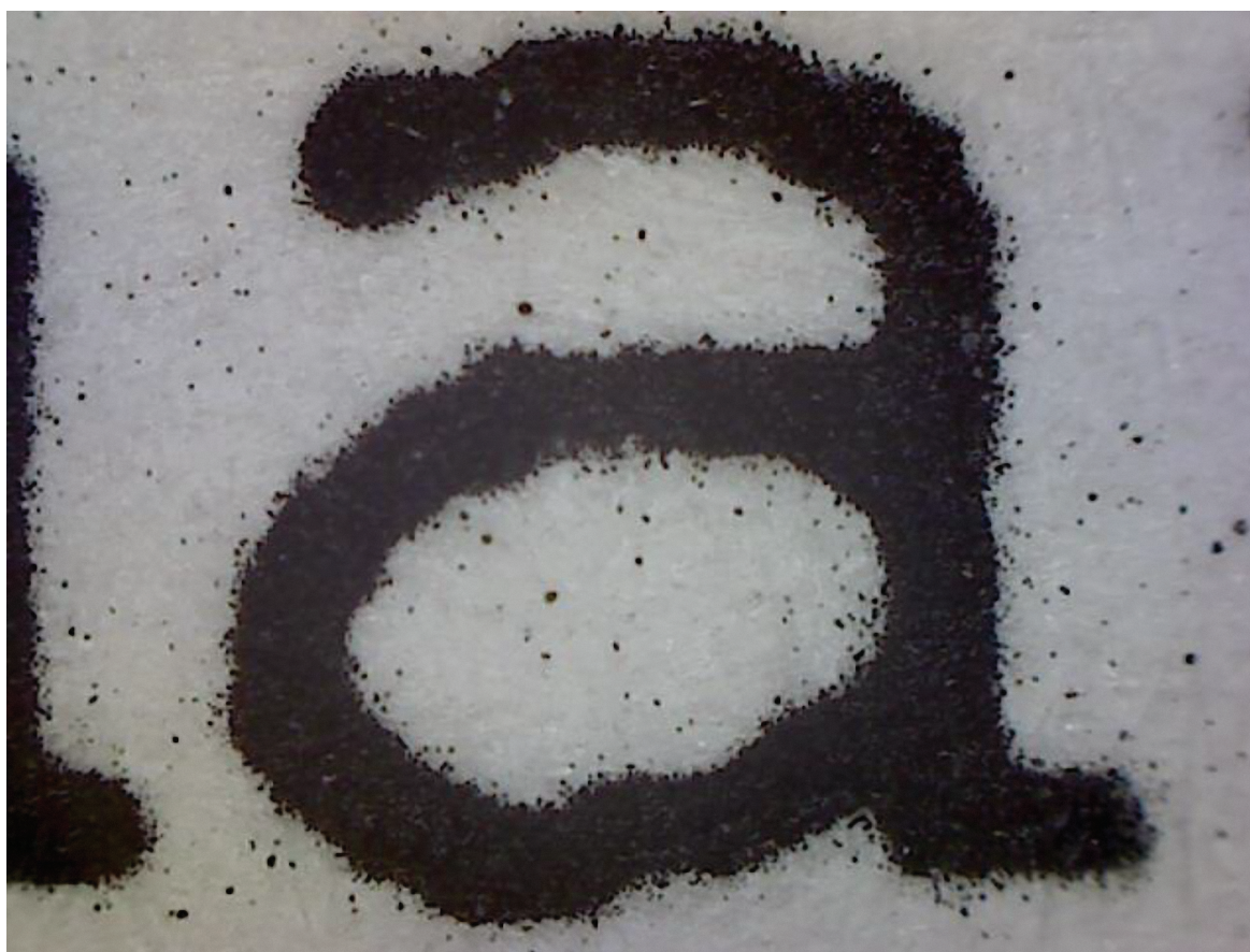
Figure 1. Toner scatter around the characters of the text printed in 1991 (photographed at 140x). The image shows an abundance of black toner particles dispersed throughout the white areas of the document—not only immediately next to the edges of the printed characters (it is termed ‘toner scatter’—a typical ‘noise’ effect occurring during the printing process) but also relatively far from them.
