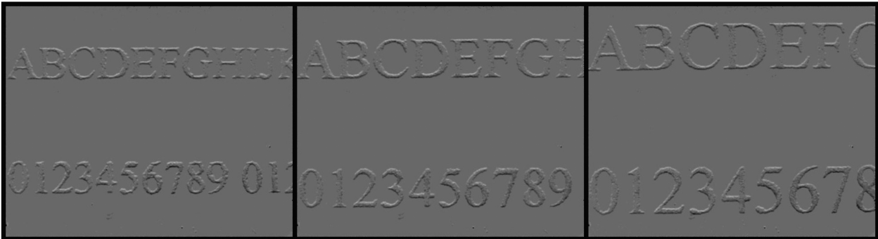
Figure 1. Standard text on which magnetic flux was measured for all phase 1 samples. 8 pt, 10 pt, and 12 pt font respectively.
