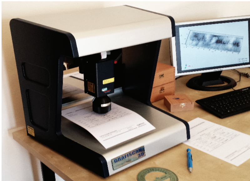
Figure 7. The Conoscan 4000 scanning system, (also called Grafiscan 3D by the author) used to perform the measurements.
