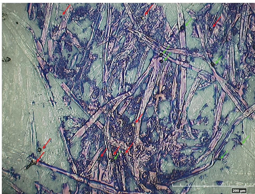
Figure 2. Handwritten stroke detail with toner particles -some particles were printed before (red arrows), others after the stroke was written (green arrow), mag. 600x.
