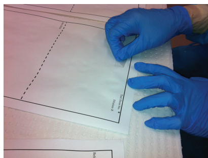
Figure 1b: Image demonstrating how to use the tape lift.
