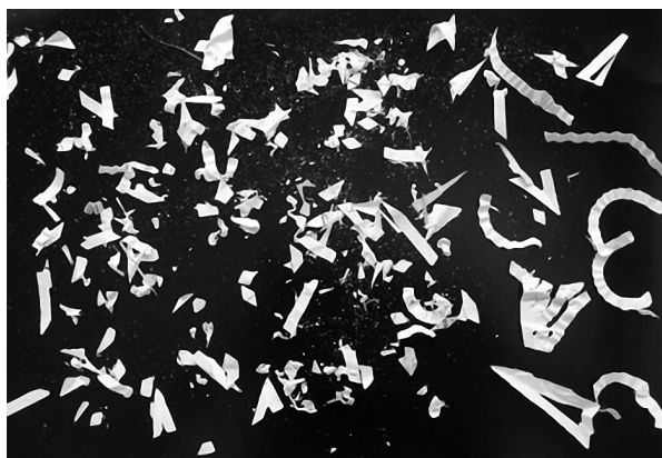
Figure 9. Debris caused from a defective strip shredder.
