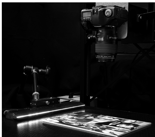
Figure 6. Raking lighting camera set-up.
