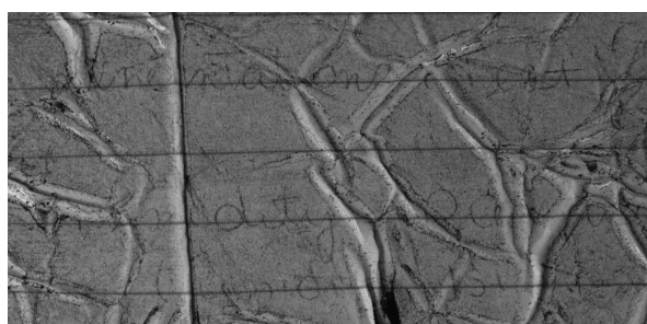
Figure 4. Image of Secondary EDD result after 80% RH and 20 lb. weight Applied.
