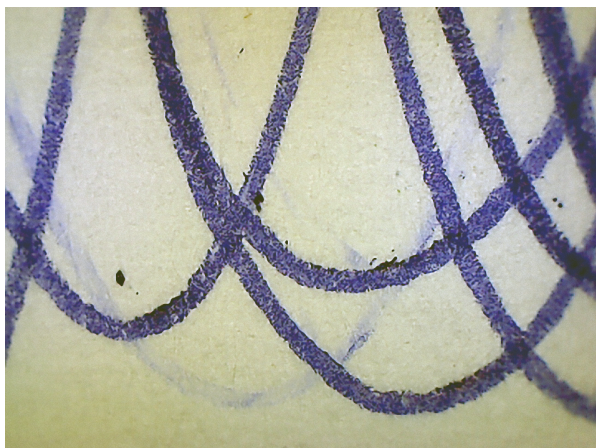
Figure 5. Long gaps present in ink strokes written with a used fine point blue ballpoint pen manufactured in South Korea (photographed at 40x). Though this pen has shown good writing characteristics when preparing multiple writing samples for this study, sometimes it produced long skips (long areas of “starving”) like the V-shaped one shown on this image.
