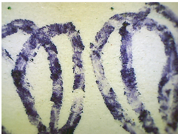
Figure 4. Multiple skips (gaps) reproducibly exhibited in the writing samples prepared with a used gift medium point blue-violet ballpoint pen (photographed at 40x). The image clearly shows a high level of malfunctioning of the pen that is not typically observed in ballpoint ink writing. In this study, such a peculiar pattern of alternating skips and areas of heavy deposits of ink was shown by only one out of the 400 pens tested.
