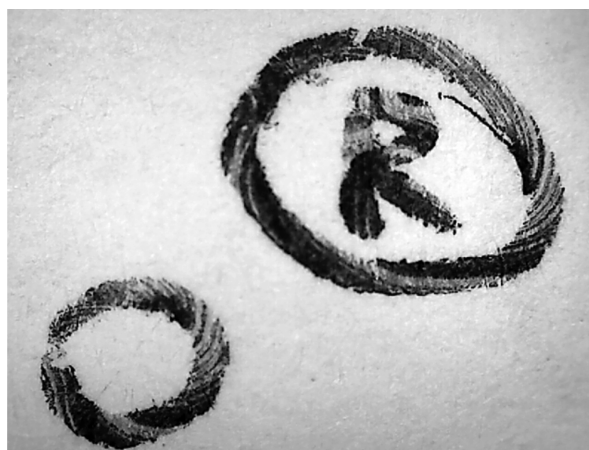
Figure 2. Elaborate striations reproducibly exhibited in the writing samples prepared with a used Bellagio® (Las Vegas, NV) medium point black ballpoint pen (photographed at 40x).
