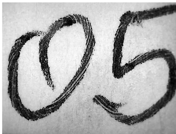
Figure 3. Elaborate striations reproducibly exhibited in the writing samples prepared with a used pharmaceutical company (Michigan, 2010) medium point black ballpoint pen (photographed at 40x).
