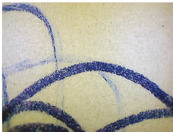
Figure 7. Two long gaps (long areas of “starving”) present in ink strokes written by a new, high-end medium point Aurora® (Italy) blue ballpoint pen (photographed at 40x).
