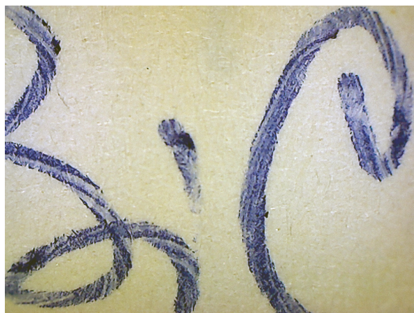
Figure 1. Elaborate striations reproducibly exhibited in the writing samples prepared with a used Bic® (Sweden, 1992) medium point blue ballpoint pen (photographed at 40x).
