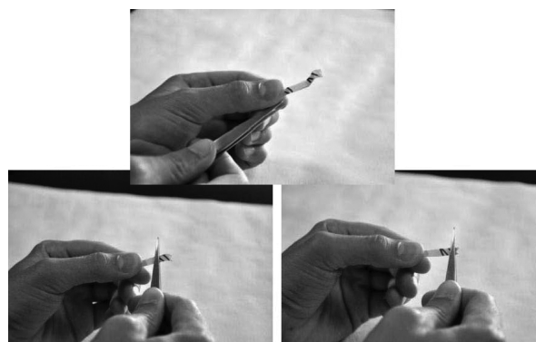
Figure 1. A bent shred being uncurled with forceps.
