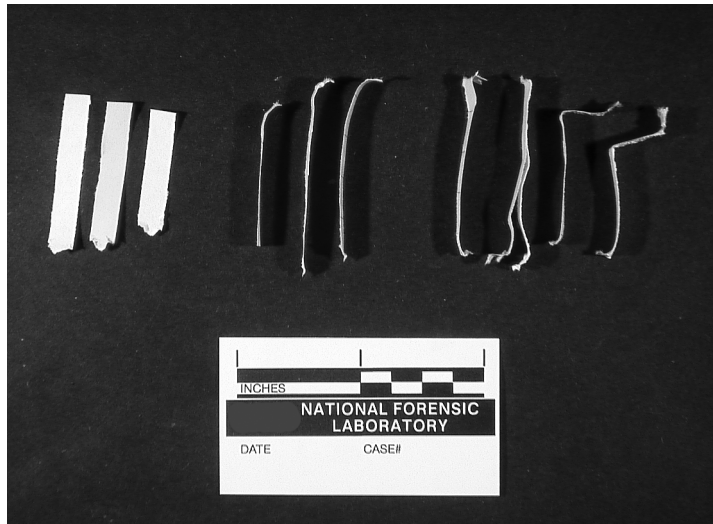
Figure 11. Curled ends on shreds from the same document, shredded by the Brinks machine: left, shreds with minimal or no curling; middle, shreds with one curled end; and right, shreds with two curled ends and/or major deformation.
