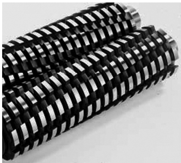
Figure 2b. Example of “negative profile” cylinders (photograph courtesy of Martin Yale Industries).
