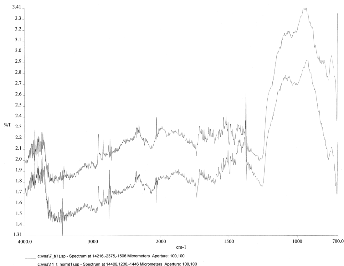
Figure 6. Comparison of the FT-IR spectra of toner-on-paper samples taken from pages 7 (upper spectrum) and 11 (lower spectrum) of the questioned document.
