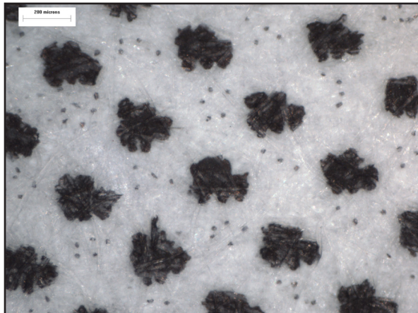
Figure 11 An example of Regular Dithering Halftone dots and their satellites revealing the quantity of drops printed by Canon bj255sp in Normal mode.
