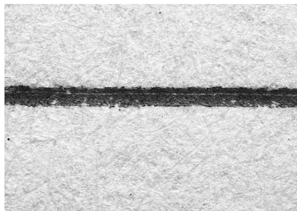
Figure 6 Liquid Lead Pencil Line Morphology
