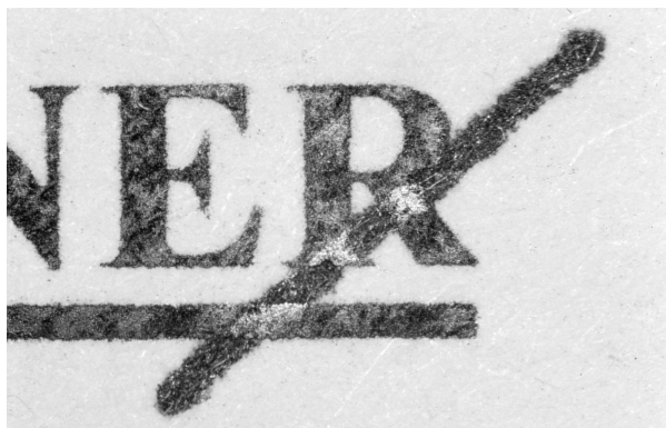
Figure 3. Reflection-enhanced macro showing characteristic glare behavior of a film of dried ink resulting from a written mark that had crossed over laser printing.
