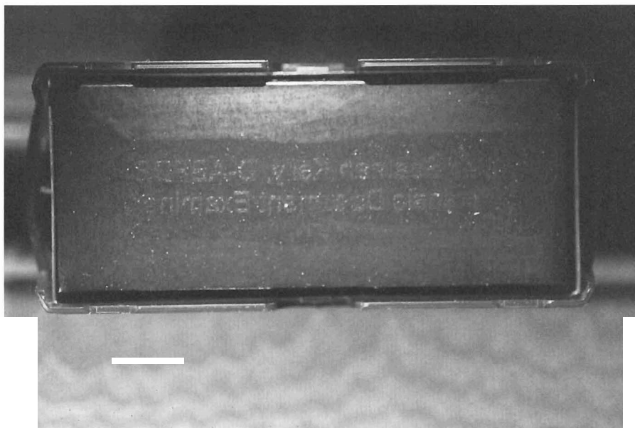
Figure 3. Image area of the SC-300 PC die is flat. Ink exits through the micro pores in the image area. The die is ink free in the non-image area.
