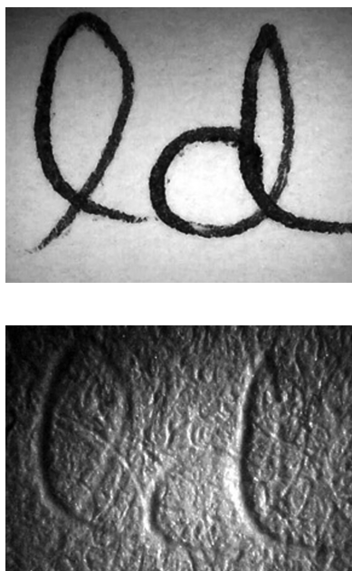
Figure 3. Ballpoint pen writings before soaking in water. The upper photograph was taken under daylight, and the lower photograph showing ballpoint pen grooves was taken with oblique infrared rays.
