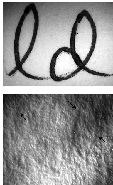
Figure 4. Ballpoint pen writings on bond paper soaked in alkaline medium for 20 days. The upper photograph was taken under daylight, and the lower photograph was taken with oblique infrared rays. Note marked decline in the intensity of grooves.
