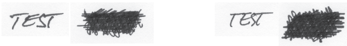
Figure 3. Sample #2 consisted of the word “test” written on plain paper using ink 1 (Sanford Uni-ball Fine) on the left, and ink 4 (Merangue Roller refill RBRF-BKB) on the right. Ink 4 was used to obliterate ink 1 (2nd image from left) and ink 1 was used to obliterate ink 4 (image on right).
