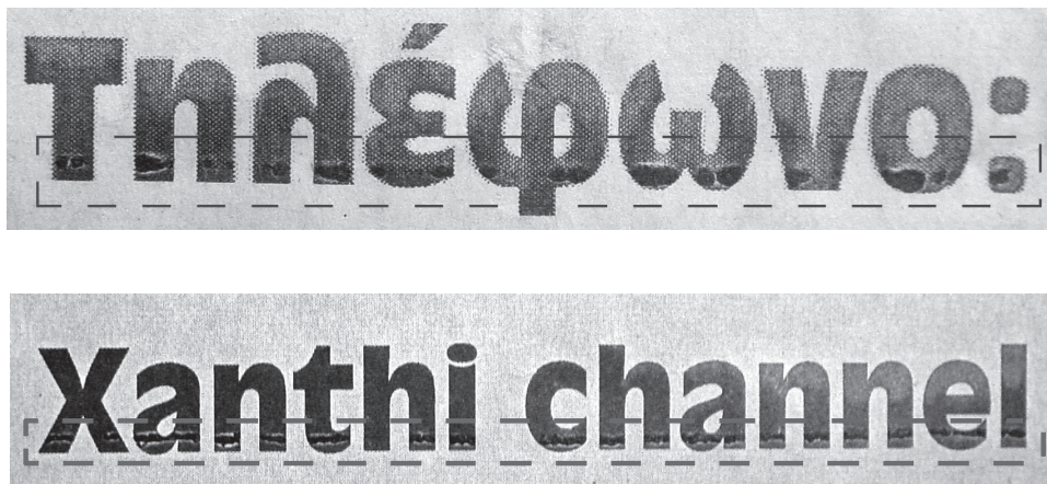
Figure 5. Printed letters in the lower half of page 1 on 2 of the 3 questioned inserts contained uneven inking (indicated by the dotted lines) for Q2 (top) and Q3 (bottom).
