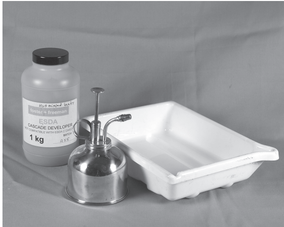
Figure 5. Cascade developer, plant mist sprayer, and plastic film tray used in the mist + humidity method.
