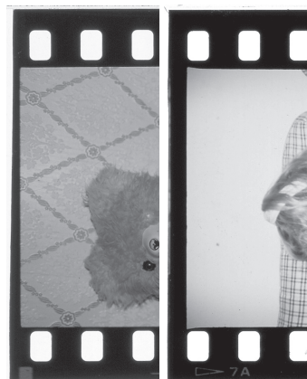
Figure 1. Examples showing differences in the position of the image frame relative to the sprocket holes.
