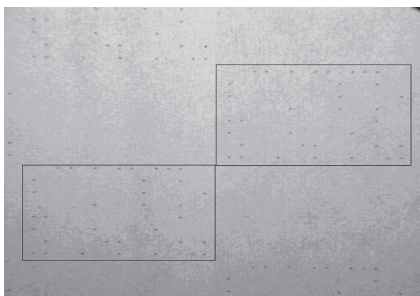
Figure 5. Arrangement of repeated dotted motifs present on a printout from Fuji Xerox DocuPrint C831 color laser printer.
