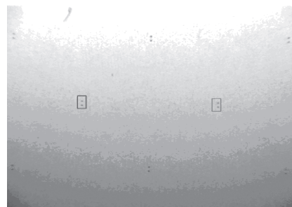
Figure 6. Arrangement of repeated dotted motifs present on a printout from RICOH AP305 C2000 color laser printer.
