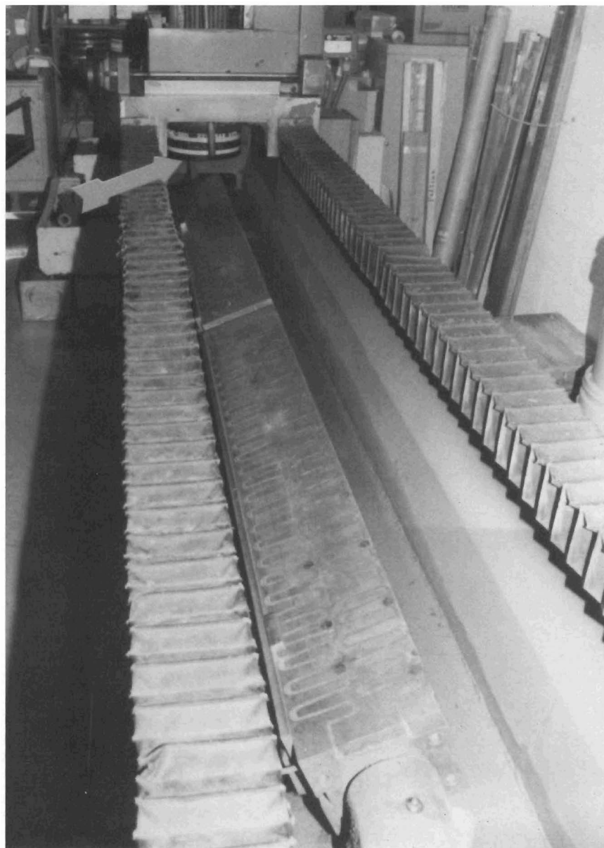
Figure 2. A rotating sharpening wheel (arrow) will travel across and sharpen the edge of the long guillotine blade when mounted in this machine.
