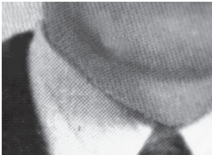
Figure 3. Discrepancies found in the alignment of printing dots resulting from a cut-and-paste in an altered passport.
