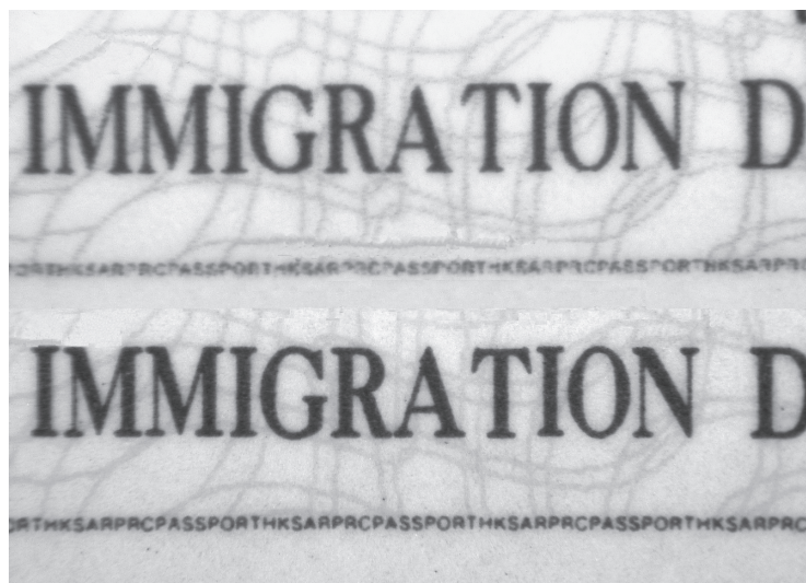
Figure 7. As a result of discrepancies in the printing quality and the printing method, nondecipherable microprinting on the questioned passport can be observed.
