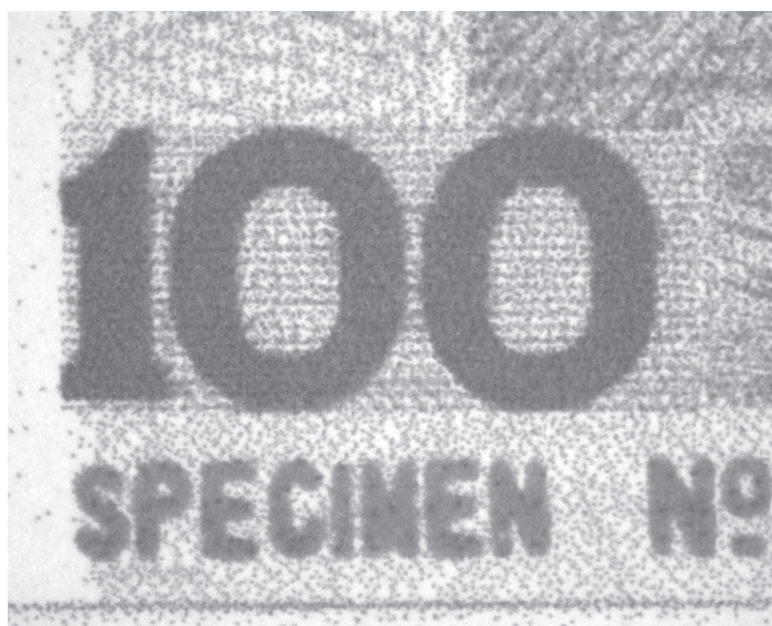
Figure 2b. Control BOC HK$100 banknote prepared from Epson Stylus CX3100 all-in-one inkjet printer.
