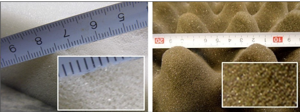
Figure 6 Left, open surface structure of the polyurethane soft foam plates. Right, special structured acoustic polyurethane foam plates.
