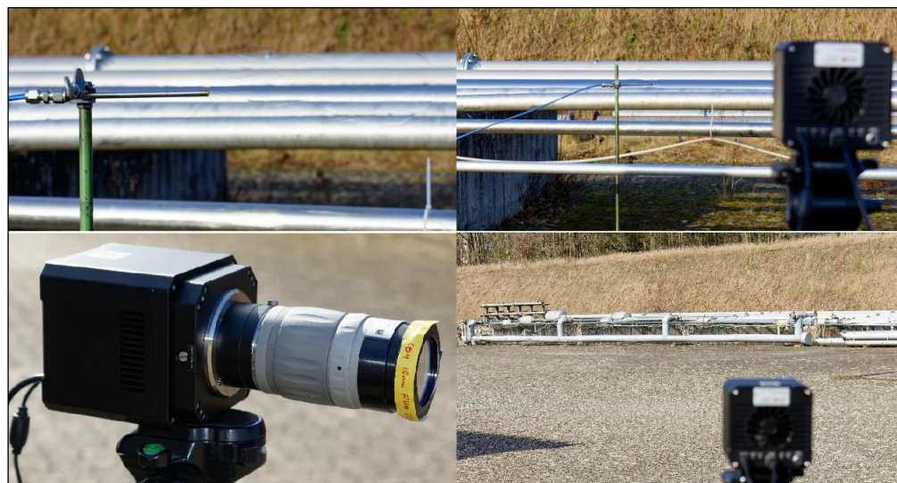
Figure 1 Top row: 50 l/min hydrogen flame (left) and UV camera setup @ 2.5 m distance (right). Bottom row: Camera system with UV filter (left) and experimental setup @ 40 m distance (right).
