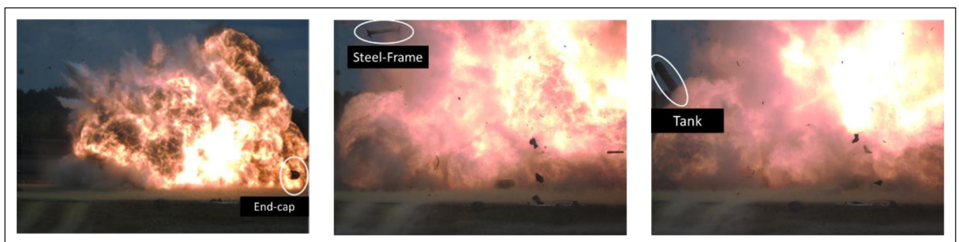
Figure 4 Test 4 – Fragments emerging from the fireball.
