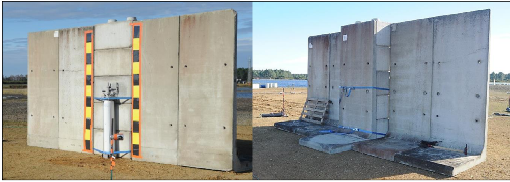
Figure 2 Concrete blocks at the back of the hydrogen tanks—left: front view with a Type I tank. Right: rear view.
