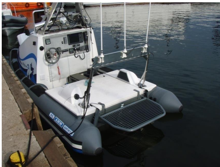
Fig. 7. Landing placed aft — place to install a launch and recovery system (design developed under the project) [4]
