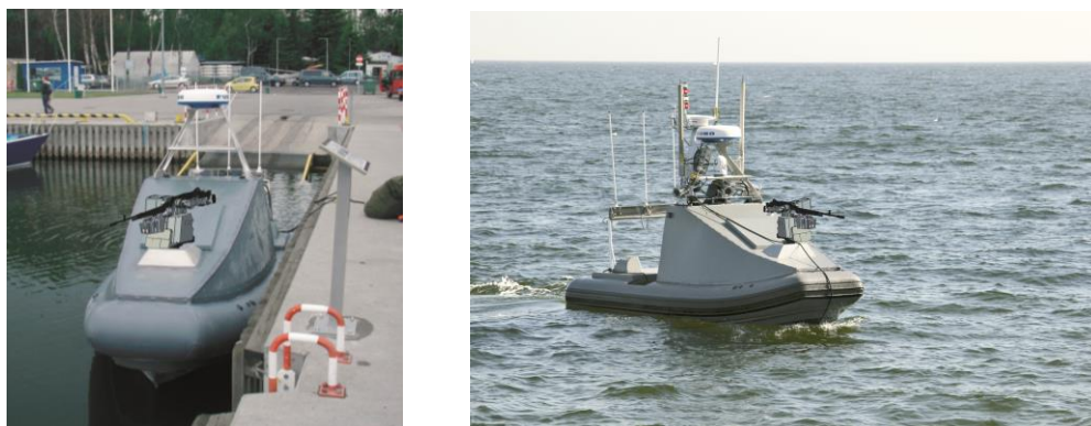
Fig. 6. USV 'Edredon' with installed weapon module (first phase of development) [4]
