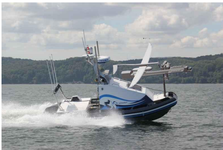
Fig. 12. USV 'Edredon' fitted with the designed small UAV pneumatic launcher [3]
