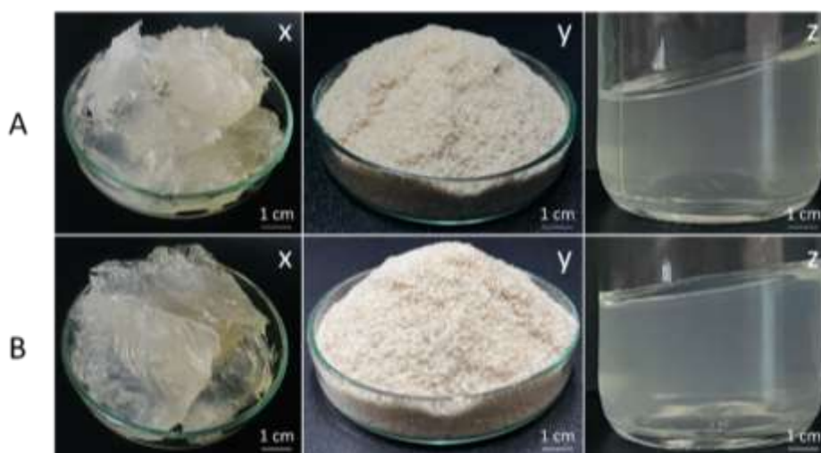
Figure 4. Production of carrageenan from Kappaphycus alvarezii : (A) Carrageenan from green morphotype of K. alvarezii , (B) Carrageenan from brown morphotype of K. alvarezii : (x) Extracted carrageenan gel after precipitation in 0.2 % KCl, (y) Dried and powdered carrageenan, (z) Set carrageenan gel from 4 % (W/V) carrageenan solution.
