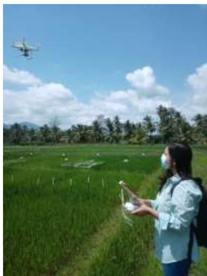
Figure 6. Capturing multispectral images using the P4 Multispectral UAV over the rice field during 1.5 month before the harvest
