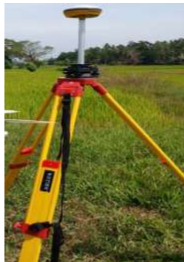
Figure 7. Real-time kinematic (RTK) GPS guidance system
