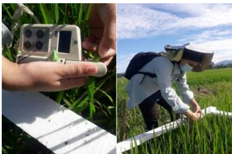
Figure 4. SPAD meter method used to measure Leaf Chlorophyll of the rice crop (used the fully expanded top leaf including the flag leaf from each sampling regiform quadrant)
