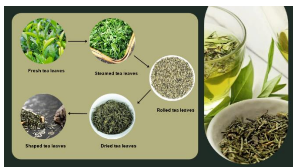
Figure 1: The appearance of tea leaves after the various manufacturing processes.
