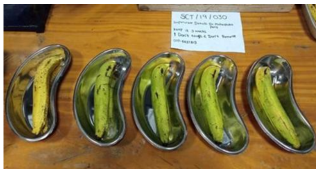
Fig. 05b. Morphology of the banana after 09 days (C0- uncoated sample, C1- coating 1, C2- coating 2, C3- coating 3, C4- coating 4).
