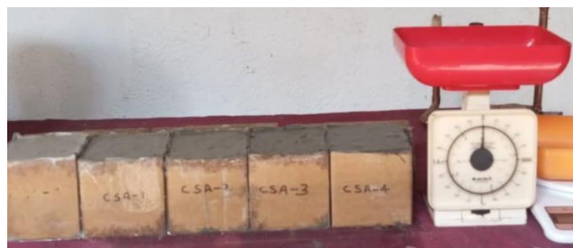
Fig. 1. 100 mm \times 100 mm \times 100 mm masonry unit specimen fabricated using ordinary Portland cement, coconut shell ash, and recycled polyester fabric reinforcement for experimental evaluation.
