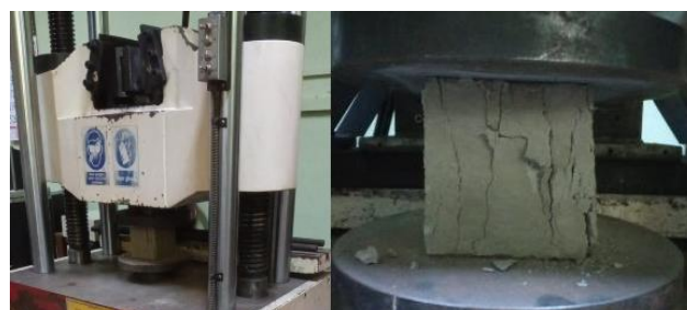
Fig. 2. Experimental setup for compressive strength testing of masonry unit specimens using a universal testing machine under uniaxial loading conditions.
