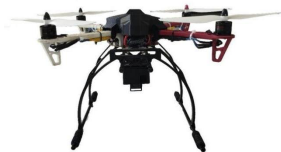
Figure 01: Quadcopter developed in the research used for image acquisition
