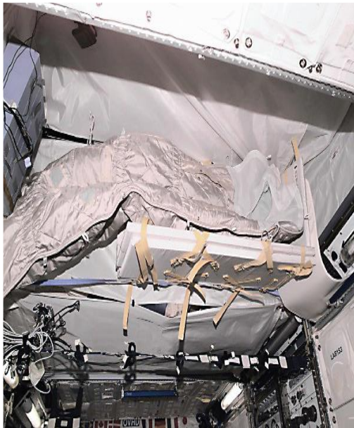
Figure 4: Temporary sleep station on the ISS with polyethylene panels and water storage above for enhanced radiation shielding (National Aeronautics and Space Administration (NASA), 2003).
