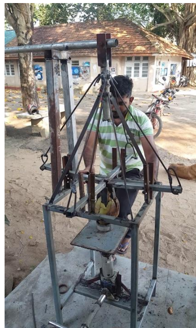
Figure 7: (a) Schematic of coconut de-husking machine and (b) constructed coconut de-husking Machine
