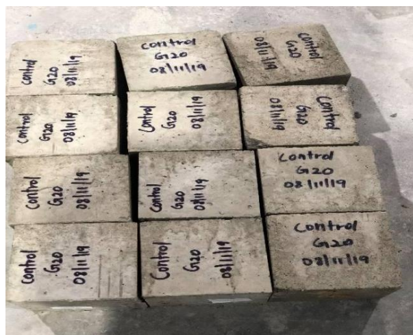
Figure 2: Hardened concrete cubes
