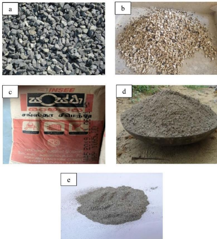
Figure 1: Raw materials. a: granite coarse aggregate b: CTCA c: OPC d: sand e: RHA
