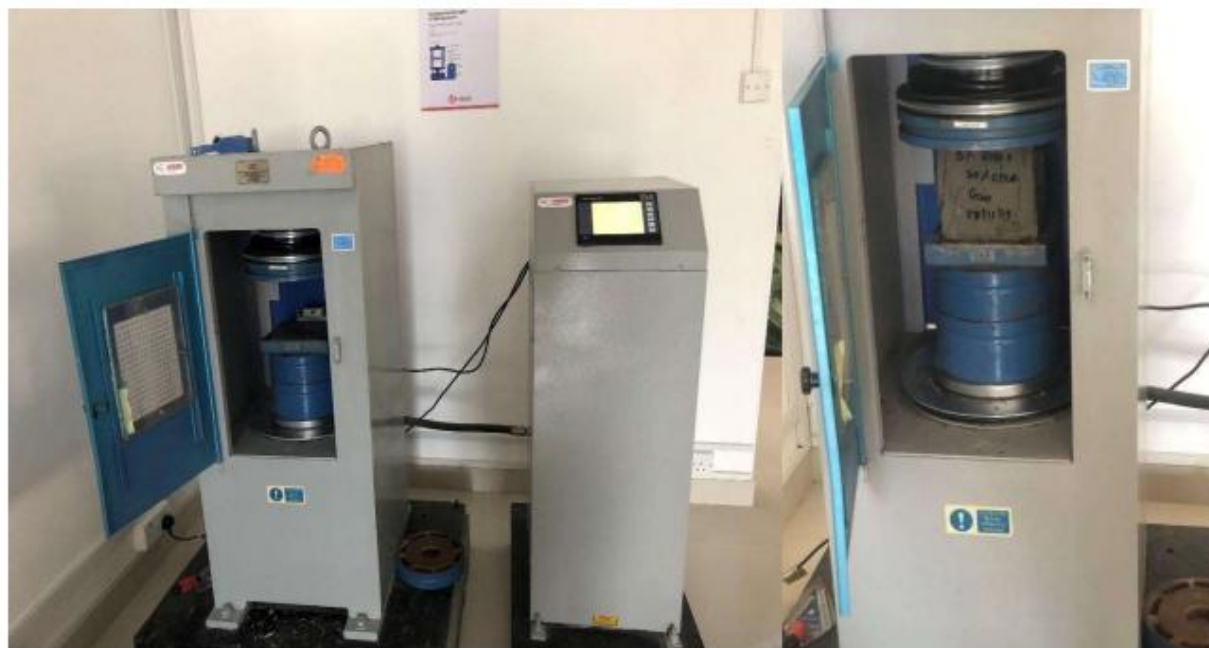
Figure 3: Equipment used for measuring compressive strength
